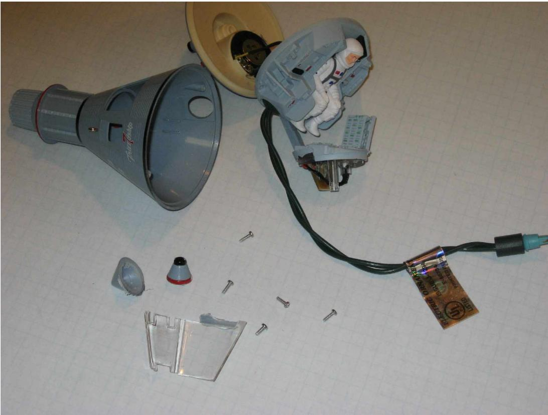
The astronaut is mounted on three little plastic pins. It should come out with a little prying. Work a small screwdriver down behind his shoulders and he'll pop out.
