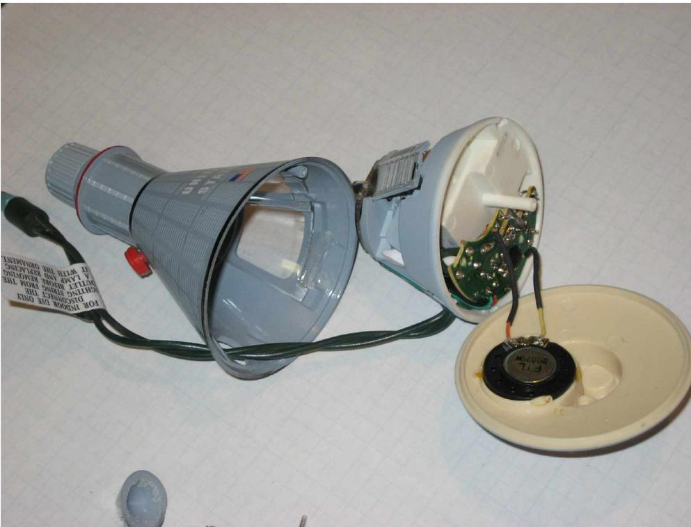
If you plan on removing the electronics, there are two screws holding the circuit board to the aft bulkhead. The instrument panel will come loose. Be careful as there are little wires going up to the button and instrument panel light.
